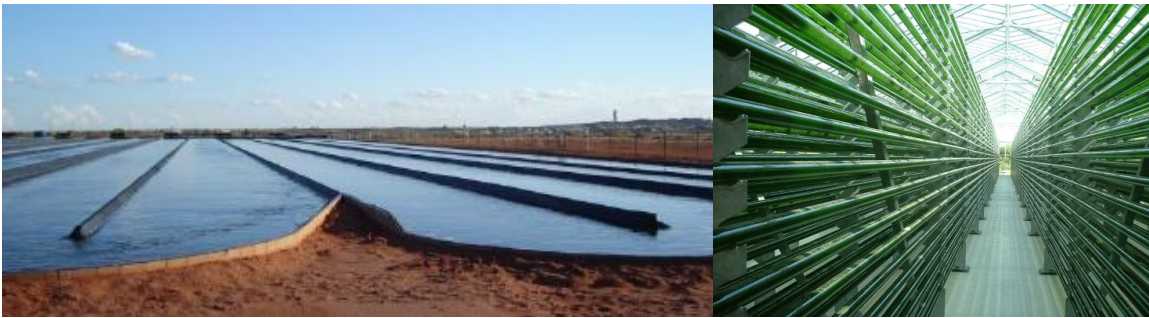
Figure 6: Algae production: open ponds (left), photobioreactors (right)
