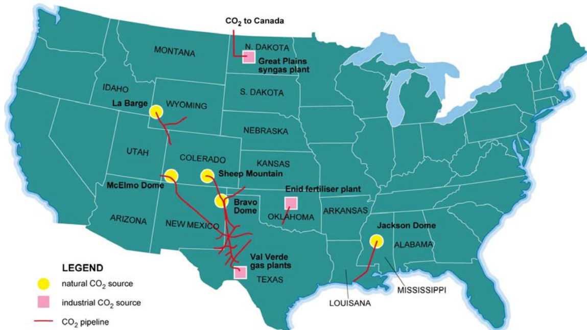
Figure 3 – CO 2 pipeline networks in the United States
